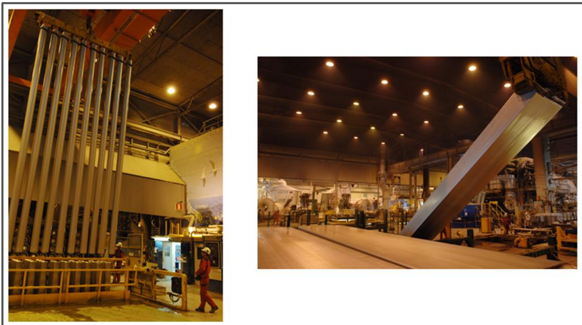
Figure 4-3 DC-cast extrusion billets (cylindrical) or rolling slabs (rectangular)
