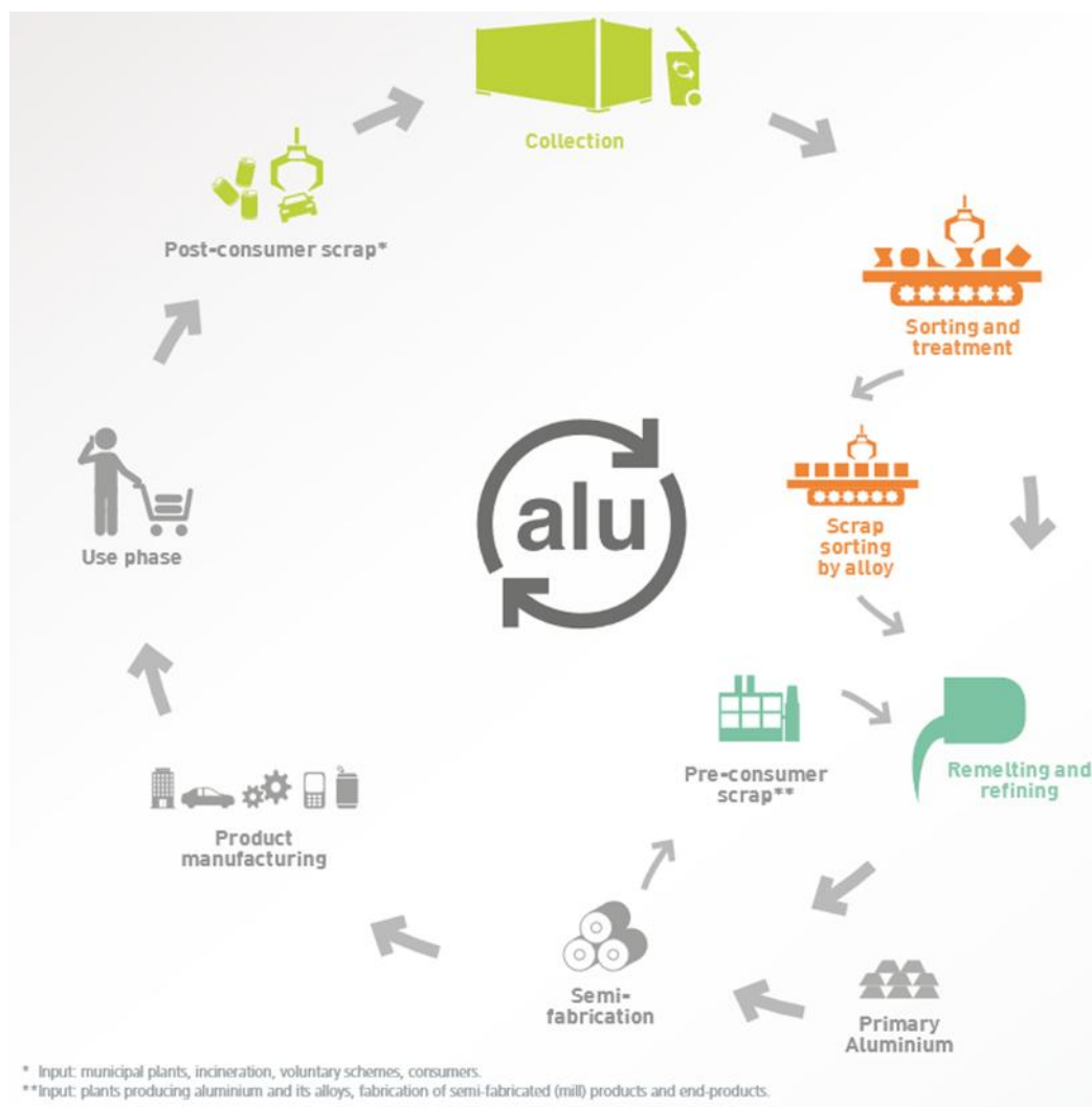
Figure 8-3 Overview of the aluminium recycling sector
