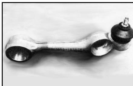
Control arm with ball bearing protected by rubber sleeve
