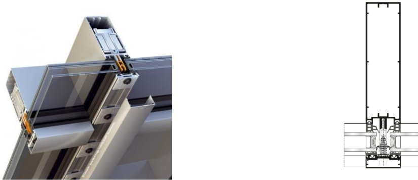
Figure 2: cross section of M50 mullion and transom
