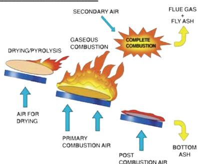
The main steps in the incineration process are pictured here in a diagram based on a similar model used by Professor Buekens of the VUB University of Brussels. Obviously modern incinerators as used in Western-Europe have to meet the highest EU environmental and health and safety standards in terms of emission controls and energy efficiency.
